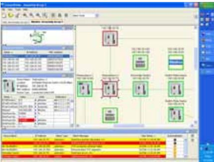
*The ConneXview workspace contains multiple task panels and displays the health of the network in colors to speed up problem identification and troubleshooting.*
