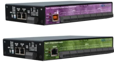
Sealevel Systems Inc., announces two additions to the popular [Seal/O family](#) of modular I/O – the Seal/O-530 and Seal/O-540 digital I/O modules. Offering a powerful selection of open-collector outputs and optically isolated inputs, the modules are designed to interface to a variety of real-world I/O. Ordering options allow control from a host device via wireless, Ethernet (Modbus/TCP), RS-485 (Modbus), USB, or RS-232.
