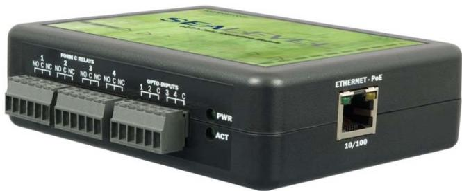
Sealevel Systems, Inc. announces the new eI/O family of Ethernet digital I/O solutions. eI/O modules provide system designers with a compact, low-cost alternative for monitoring and control and are perfect for a wide variety of applications including process control, facility management, security, and broadcast automation.
