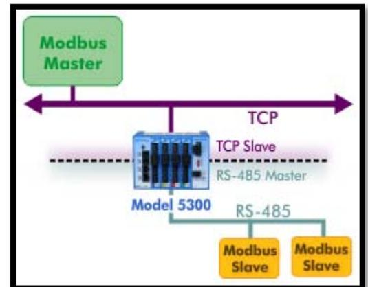
*The Model 5300 can serve as both a master and slave on different networks that are connected. In this diagram the 5300 is a slave on the TCP network and a master on the RS-485 network.*
