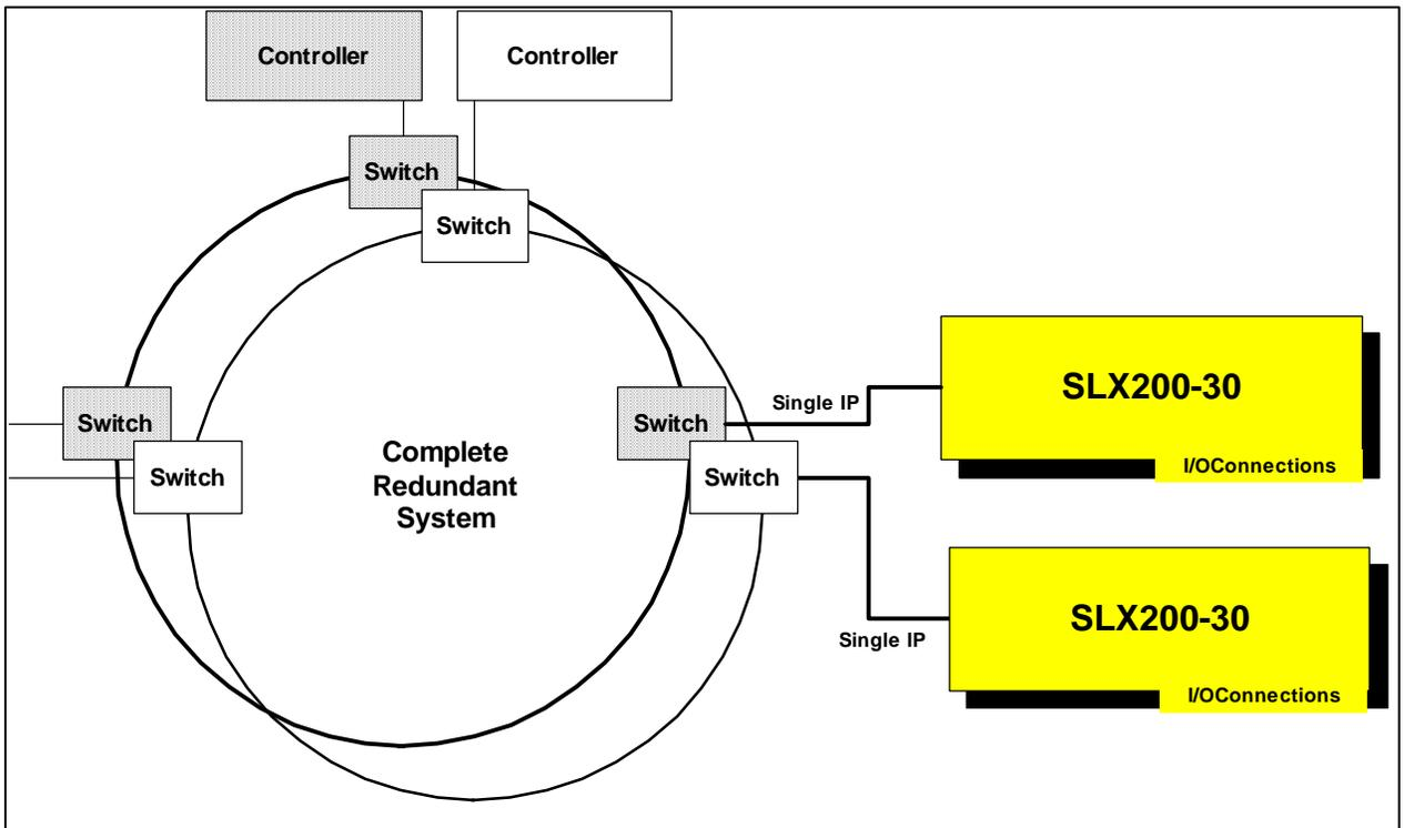
As shown in these graphics, it is no longer necessary to spend time searching for lost data as simple yet very effective methods of redundant data acquisition are readily available. Dataforth's isoLynx<sup>®</sup> SLX200-30 is a highly efficient redundant Ethernet data acquisition system that is usable across all types of redundant configurations.
