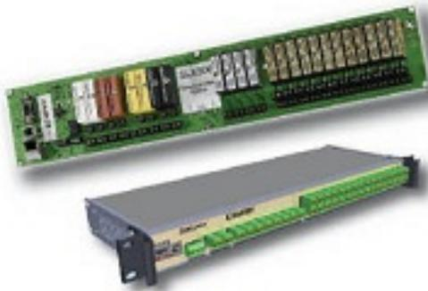
Using industry standard Modbus RTU or TCP protocols, the 8B isoLynx® SLX300 enables communication with a broad range of existing third-party software tools and HMI/SCADA packages. Pluggable modules provide the system with maximum flexibility of analog and digital channel configuration (choose from 70 analog and 14 digital I/O modules), making it ideal for factory automation, process control, test and measurement, machine control, and data acquisition applications.
