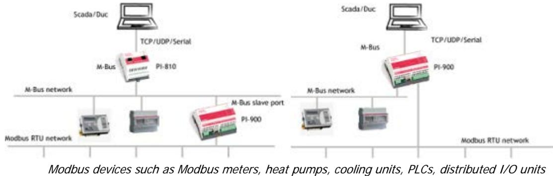
**PiiGAB M-Bus 900 is a M-Bus gateway/converter developed to enable energy optimization for buildings, industries and within energy production. Now, we release a new unique application for the PiiGAB M-Bus 900, named **Modbus2Mbus**! This application enables communication via M-Bus with Modbus units on your existing M-Bus network. Exactly as the name reveals, you can now get your Modbus values into M-Bus!**
